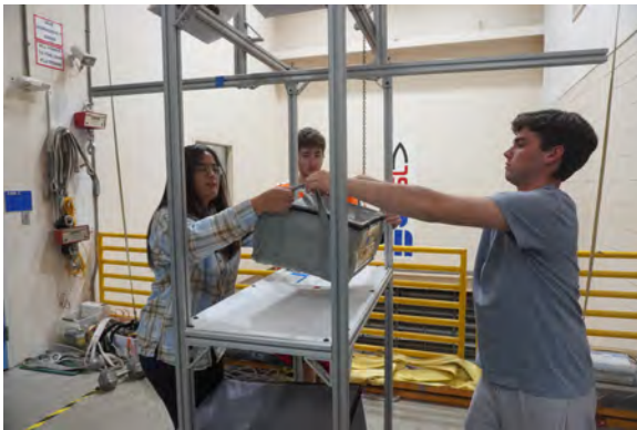
Figure 4. Testing CTB transfer with direct handoff through Cygnus hatch
