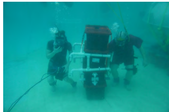
Figure 19. Two-subject manipulation of 400 kg inertial mass module (627 N/141 lb lunar weight) under simulated lunar gravity
