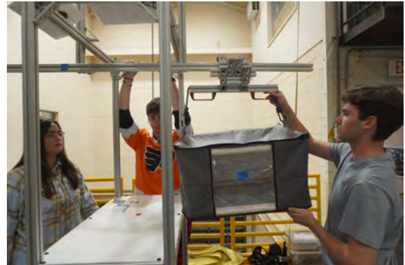
Figure 5. Testing CTB transfer using rail transport system through Cygnus hatch
