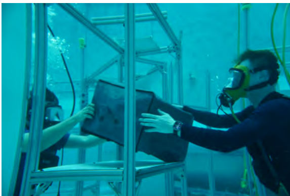
Figure 11. Passing large CTB through upper 1m x 1m portal
