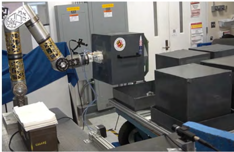
Figure 24. Robotic manipulator removing SPLC mockup from trailer mount prior to installation into suitport (half scale) 13
