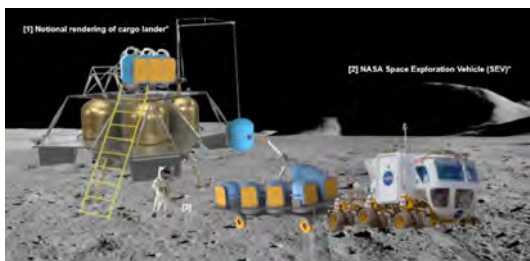
Figure 16. Offloading of SPLC modules from lunar lander onto trans-port trailer 13
