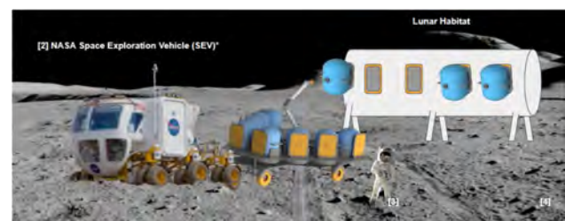
Figure 17. Station transport trailer at habitat for installation and removal of SPLCs 13
