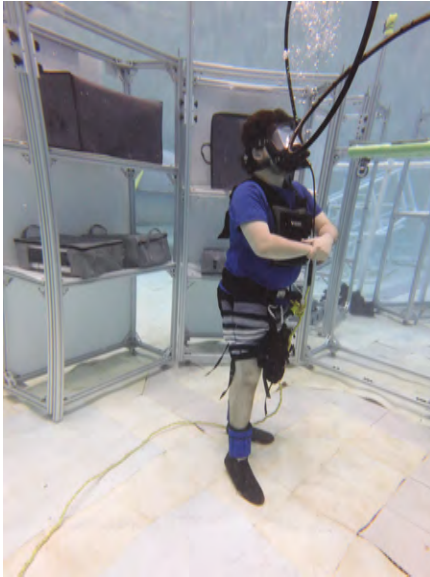
Figure 9. Underwater test subject ballasted to lunar gravity with racks containing CTBs
