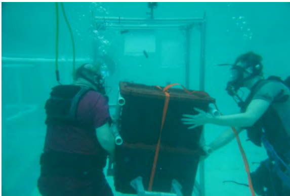
Figure 18. Two-subject installation of 200 kg inertial mass module (314 N/70 lb lunar weight) in mockup suitport under simulated lunar gravity
