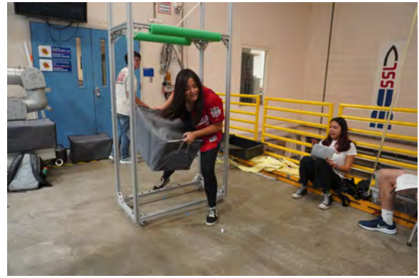
Figure 3. Testing CTB transfer with walkthrough hatch
