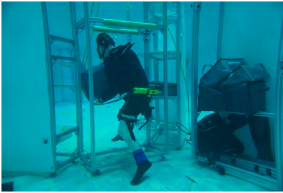
Figure 13. Carrying CTB through 1.5m x 1m portal (solo transfer)
