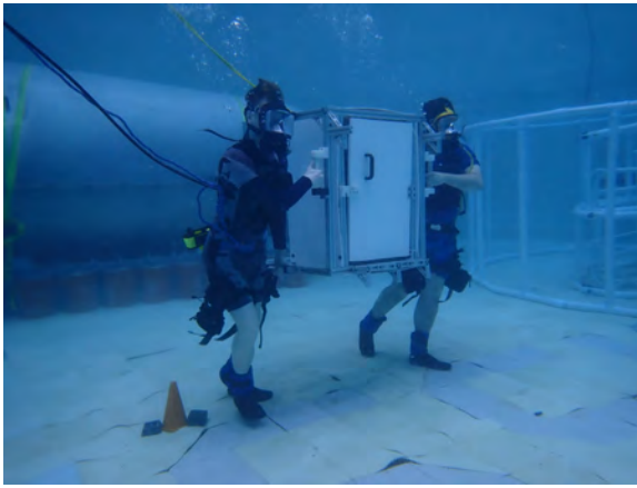
Figure 22. Transport of higher fidelity SPLC mockup under simulated lunar conditions
