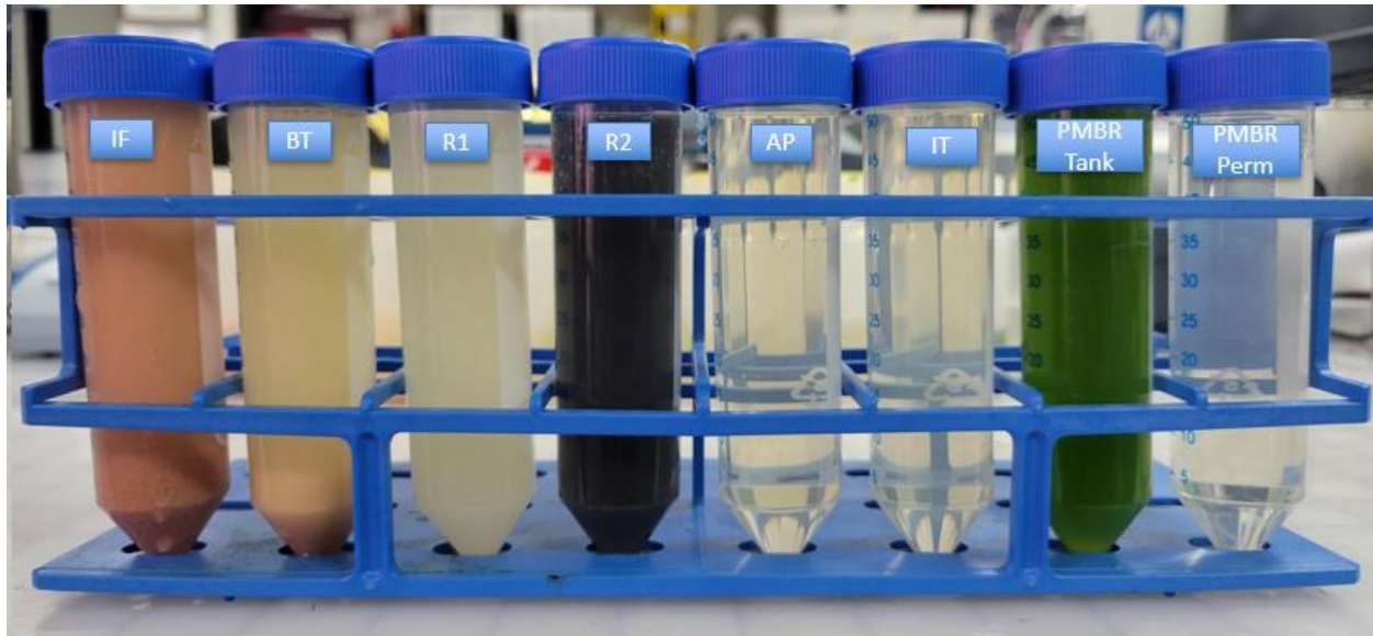
Figure 3. APMBR Samples pre-centrifugation. From left to right: Influent tank (IF), Buffer Tank (BT), Reactor Tank 1 (R1), Reactor Tank 2 (R2), Anaerobic Permeate (AP) Intermediary Tank (IT), PMBR tank, and PMBR Permeate (PP).
