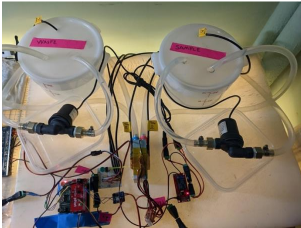
Figure 4. Development of prototype of WASTE reservoir and SAMPLE reservoir for the Space Fermentation Chamber. Copyright 2021 by MIT SEI.
