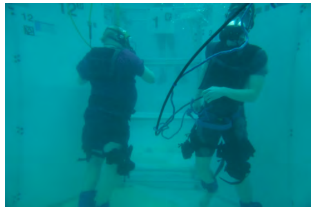
Figure 2. Test subjects wearing body segment parametric ballast to simulate lunar weight. Weights are located on the chest, upper back, thighs, and ankles.
