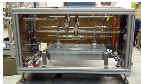
Figure 4. Carbon Dioxide Extraction Assembly. CDEA and HEA are physically identical with the exception of the membrane material.
