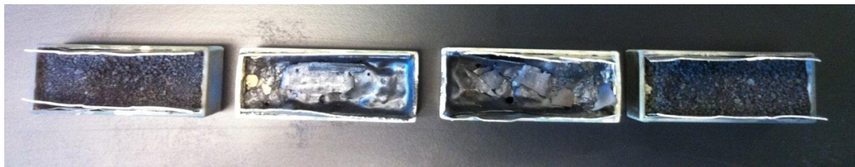
Figure 12. Sintered regolith simulant bricks. Variations in sintering observed as a result of position in high temperature furnace.
