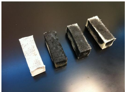
Figure 14. Polyethylene-bound regolith simulant bricks. Uneven discoloration indicates uneven temperature distribution in the furnace.
