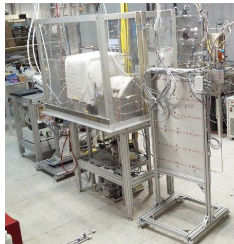
Figure 3. S-Bosch Test Stand. As assembled, the test stand includes the FFCA, RWGSRA, FRVA, WSA, and FAA.
