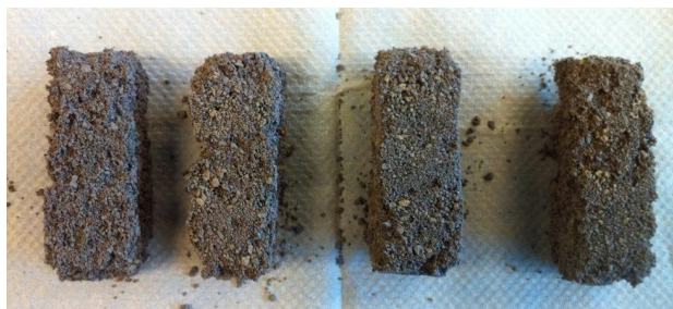
Figure 13. Sulfur-bound regolith simulant bricks. Rapid sublimation of the sulfur resulted in brittle and friable products.
