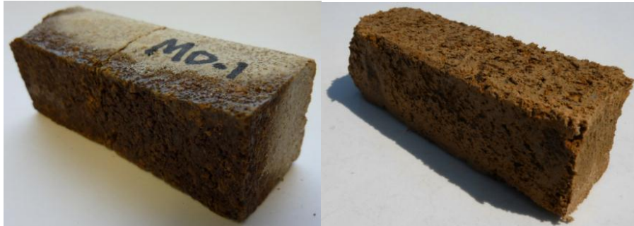
Figure 15. Martian regolith simulant brick before (left) and after (right) edge shaving.
