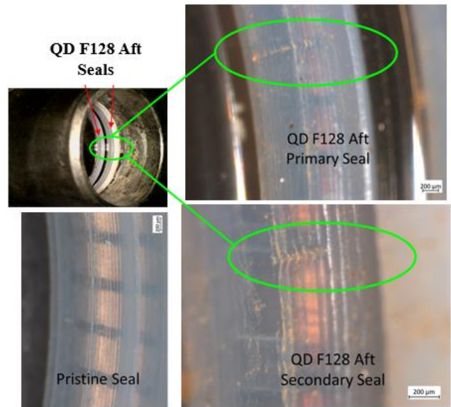
Figure 5. QD F128 Aft Seals Defect Compared to a pristine Seal (QD).
