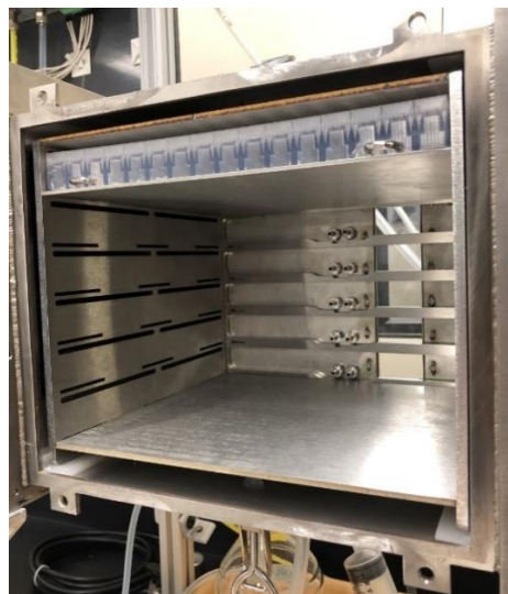
Figure 4. Sheet Metal Rack for Horizontal Contactors inside housing. Luer lock quick disconnects and airflow channels can be seen.
