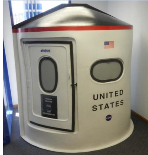
Figure 4. Earth based capsule for human factors lighting experimentation.
