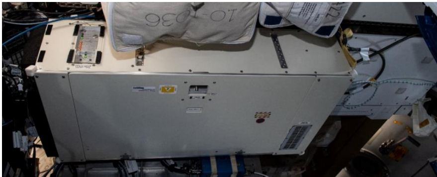
Figure 7. Brine Processor Assembly Installed on ISS.
