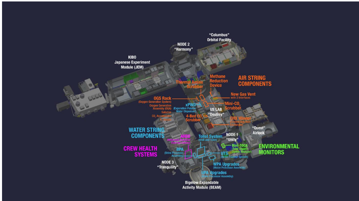
Figure 9. Exploration ECLSS Hardware Layout on ISS.
