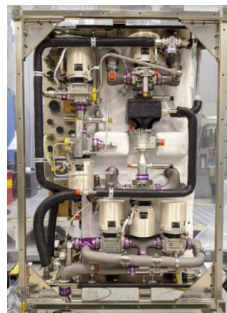
Figure 2. Four Bed CO 2 Scrubber Flight Hardware
