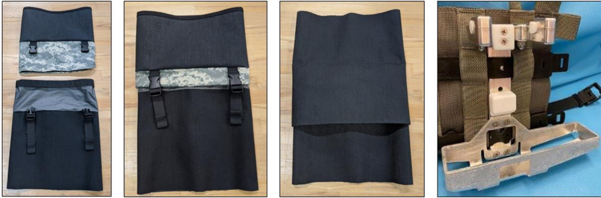
Figure 5. Attachment concepts under consideration. Prototype demonstrating a proposed roll top concept for the arm to shoulder attachment. Left: Shoulder prototype above, arm below; Left Center: Two skirts are aligned and rolled together, and structural webbings are secured with clips; Right Center: Outer skirt is lowered covering attachments; Right: Tool holster with molle webbing
