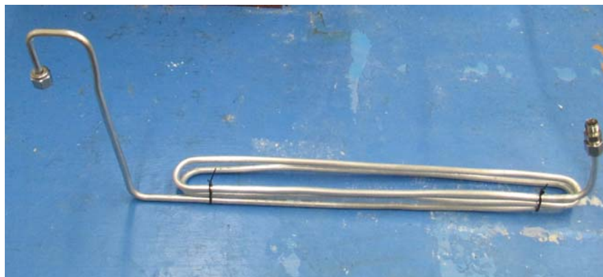
Figure 6. Temperature conditioning coil used to bring the gas temperature to that of the sorption bed.
