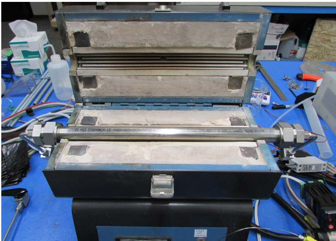
Figure 8. Thermal desorption is accomplished by heating in a tube furnace to 250°C while in a relative vacuum of <10 Torr (13 mbar).
