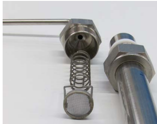
Figure 5. This image shows an expanded view of the screen and spring.
