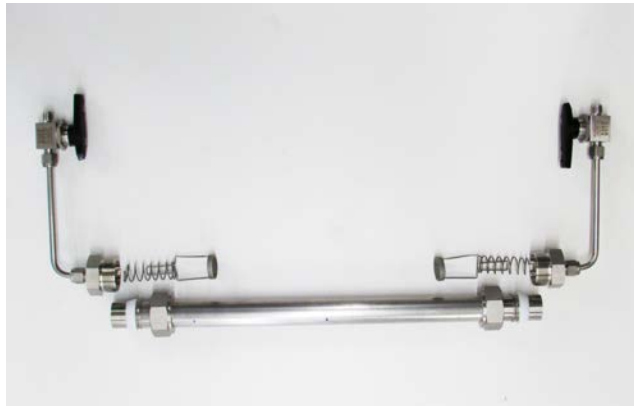
Figure 4. This image shows a disassembled bed housing.
