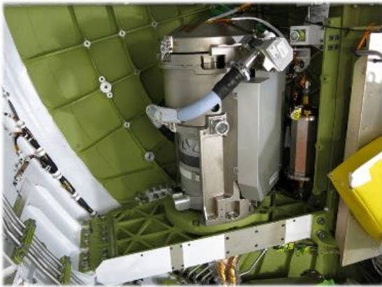
Fig. 1. Orion UWMS installed in Artemis-II Vehicle.
