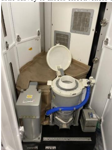
Fig. 11. ISS Acoustic Cover Prototype fit-check with UWMS Trainer in JSC's Space Vehicle Mockup Facility (SVMF), building 9
