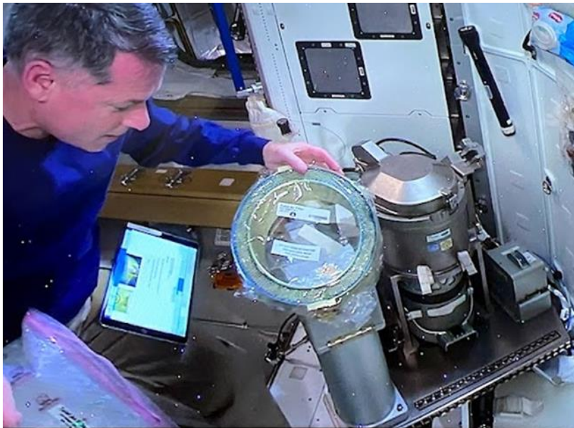
Fig. 10. UWMS with new OBF for installation.
