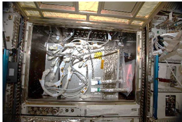
Figure 2 Technological demonstrator apparatus of JAXA water recovery system installed in Multipurpose Small Payload Rack in the ISS. ((c) JAXA)
