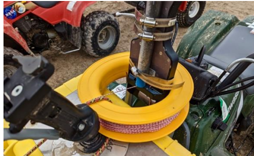
Figure 5. ATV Tethered Balloon System Interface. Close-up of ATV tethered balloon boom attachment. (HMP).
