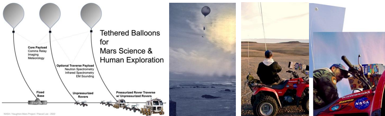
Figure 1. Concepts of Operation and Early Fieldwork on Tethered Balloons for Mars Science and Exploration. Left: Mars tethered balloon science and exploration concepts of operations at a fixed base and on mobile platforms 1 ; Center: Mars analog fixed base tethered balloon imaging experiment in 1988 at Dumont d’Urville Station, Antarctica 1 ; Right: Mosaic of HMP-2000 Mars analog ATV-tethered balloon imaging experiment 1 . Note the TV display mounted on the ATV console, with an oatmeal carton serving as makeshift sunshade (HMP-2000/P.Lee).
