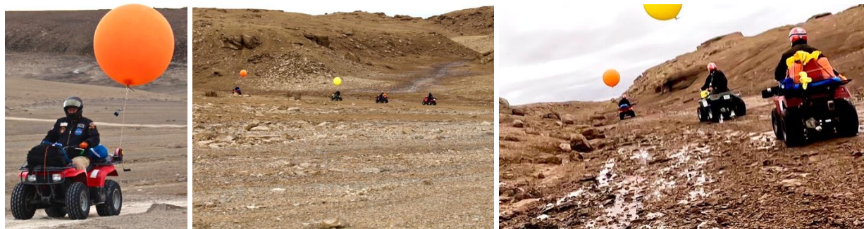
Figure 3. HMP-2022 Tethered Balloon Long-Range Traverse Experiment: Left: ATV with balloon in free tether configuration, i.e., with the tether line rising freely from the ATV-anchored reel. Note also the small black camera payload suspended from near the top of the balloon tether line. Center and Right: ATVs on traverse, two equipped with tethered balloons in free tether, entering Pete Conrad Valley shortly after departing HMP base (HMP).
