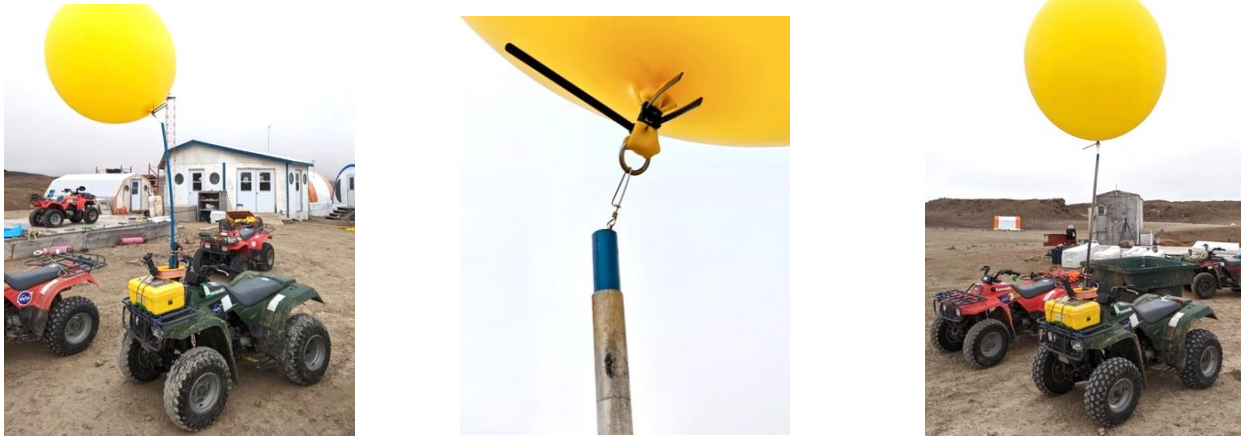
Figure 4. Iterating on the ATV Tethered Balloon System Anchor Interface: Left: ATV equipped with front-mounted blue vertical flexible PVC tube to anchor the balloon well clear of the ground when the tether line is reeled in. The flexible boom, however, interfered adversely with vehicle operation. The problem was solved by rigidifying the boom. Center: To increase boom rigidity, the blue PVC tube was inserted through a rigid steel tube to reinforce it. Right: ATV equipped with front-mounted rigid vertical boom serving as an elevated fixed anchor. (HMP).
